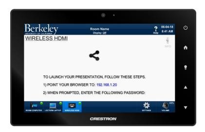
1. Press "WIRELESS HDMI" icon from home menu or toolbar to display content from your device using wireless HDMI presenter on the display.
