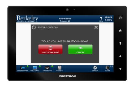
1. Press the, button on side of the touch controller to display shutdown page.
